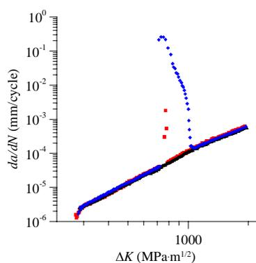
Effect of hydrogen on fatigue rate
