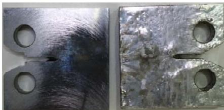
Compact tension specimens for H<sub>2</sub> testing
